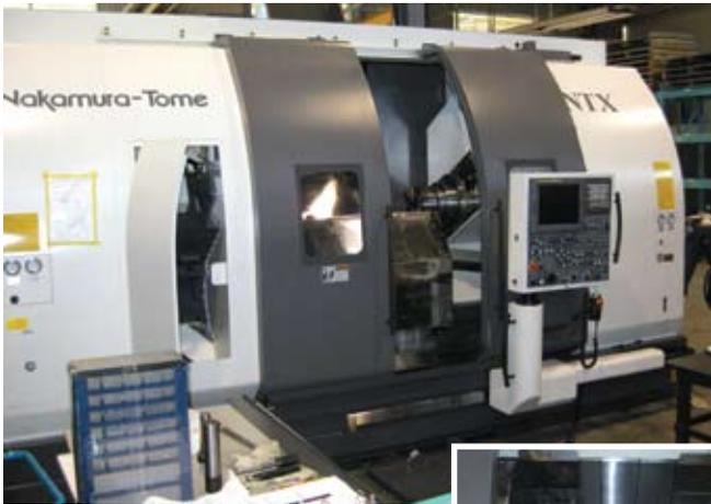
About two thirds of E. Brace's products are now manufactured on the Nakamura Tome machines. Above is the SUPER NTX model, one of three multi-tasking machines the company has installed in the past 14 months.
