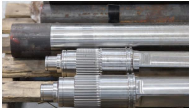
Splined shafts were produced on the Nakamura-Tome lathe.
