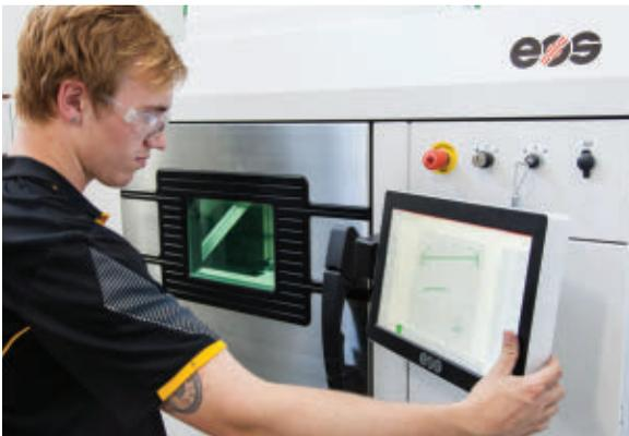
Daniel Adams, programmer and operator, initiates a build on the EOS M 290 direct metal laser sintering (DMLS) machine.
