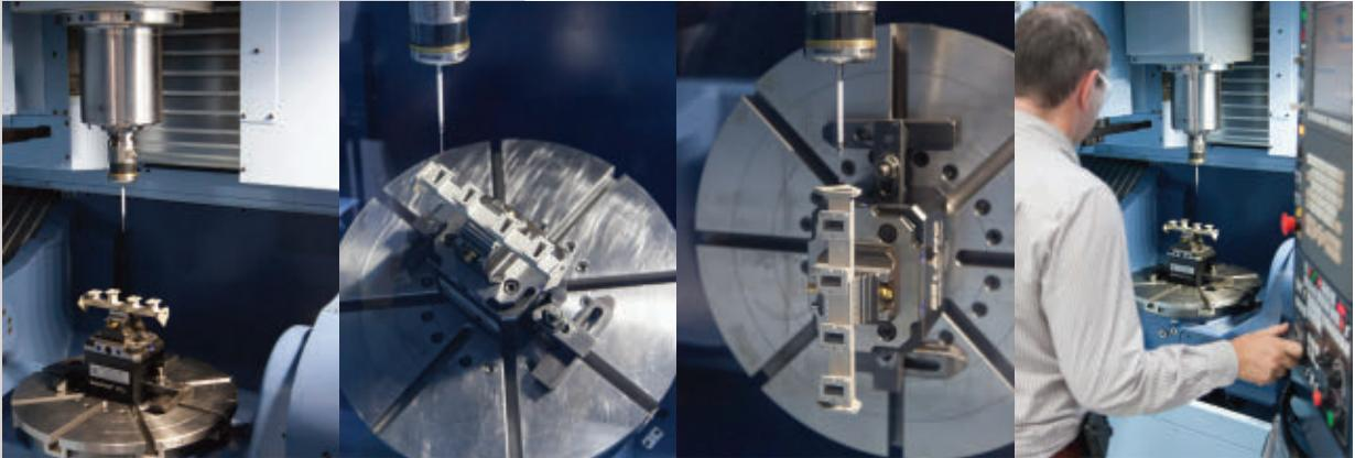
Measurements taken by a Renishaw probe are used with the CAD geometry to automatically determine the best position of the part for efficient machining in a Matsuura 5-axis mill.
