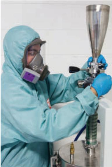
Mark Belframe, a mechanical engineering co-op student, empties a canister of used titanium powder into a sieve that will separate reusable material for recycling. Ninety-nine percent of powder not fused into a part can be used for another build.
