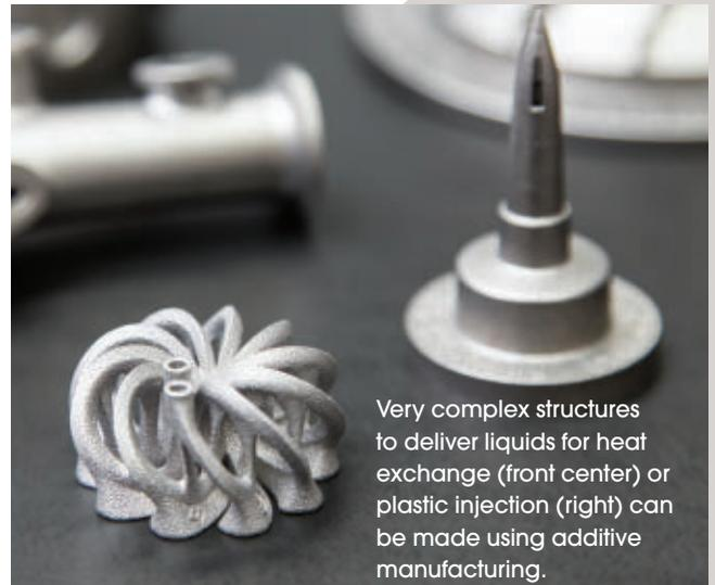
Very complex structures to deliver liquids for heat exchange (front center) or plastic injection (right) can be made using additive manufacturing.
