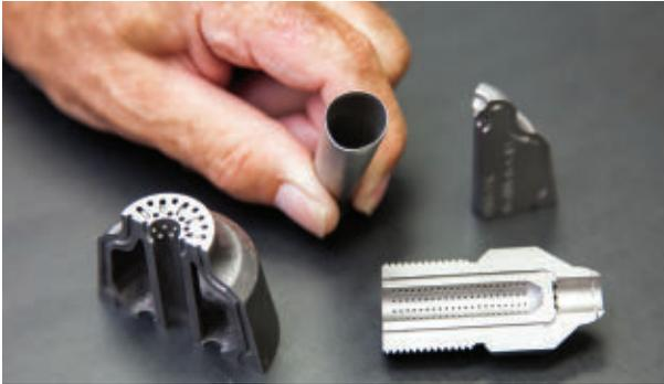
Additive manufacturing can create parts with very thin, strong walls like the one being held. A cross section of a die insert shows conformal cooling channels that mirror the shape of the die to allow for faster cooling.
