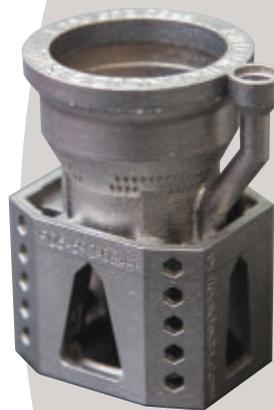
A highly complex aluminum aerospace component incorporates exacting internal and external details possible with additive manufacturing.
