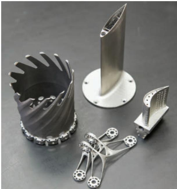
Aerospace parts built by an additive manufacturing process can weigh substantially less yet maintain structural integrity like the part in the front. Additional functionality can also be incorporated into a part's internal structure to improve fluid mechanical performance.
