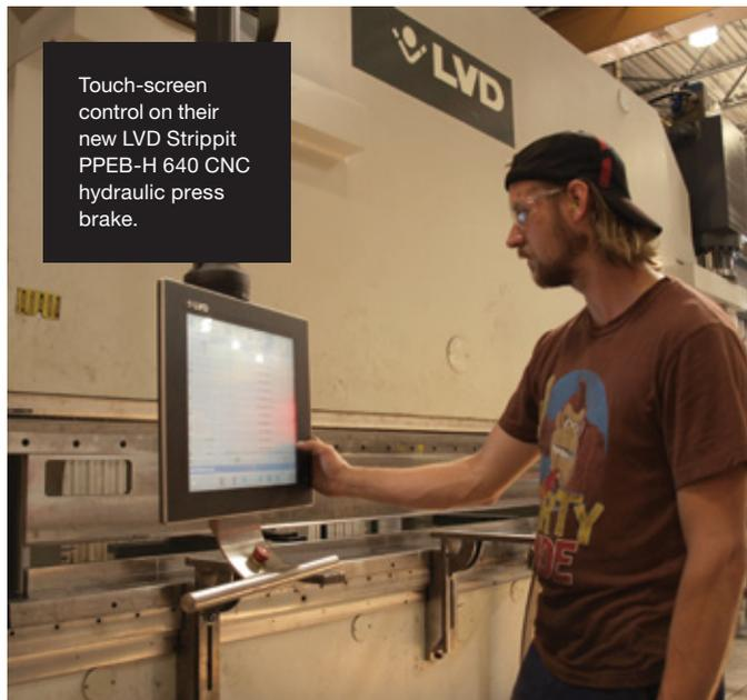
Touch-screen control on their new LVD Strippit PPEB-H 640 CNC hydraulic press brake.
