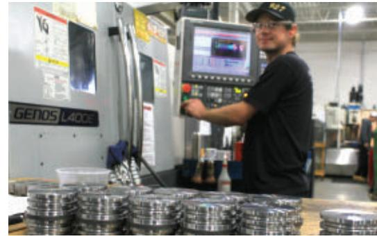
Jason Brown makes rollers for a Valiant conveyor line on an Okuma L400E CNC lathe.
