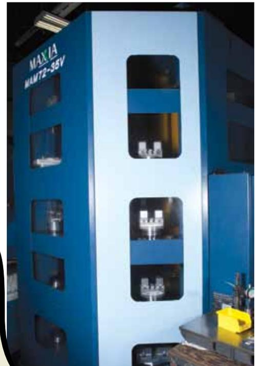
The Matsuura machining centres are equipped with pallet stocking towers.
